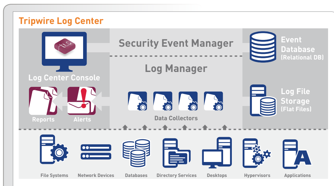
FIG. 7 Tripwire Log Center collects activity logs from anywhere in the IT infrastructure, compressing, encrypting, indexing and storing them quickly into flat files. Plus, Tripwire Log Center's security event management capabilities helps reduce security risk by getting near real-time dashboard visibility to security events and correlating events of interest, alerts and vulnerability data.
